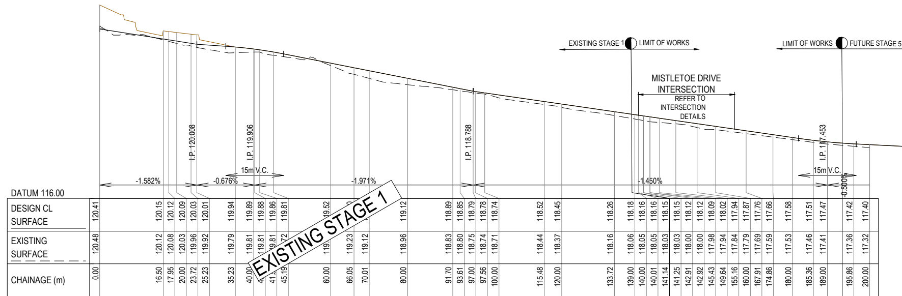
EVERLASTING BOULEVARD - LONGITUDINAL SECTION
